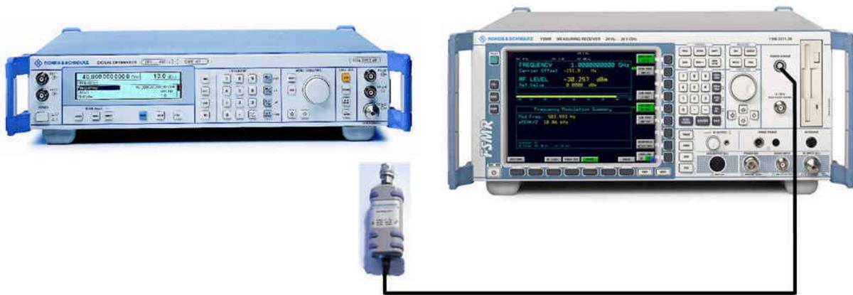
Fig.2-2 RF Power measurement setup
