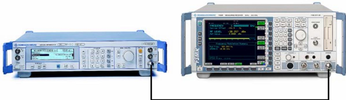
Fig.2-9 AM modulation measurement setup
