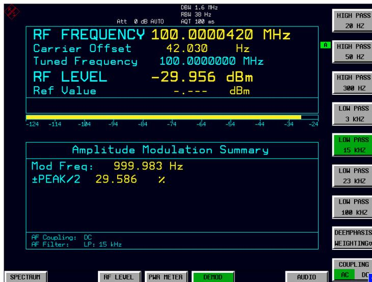
Fig.2-10 AM Modulation measurement in the DEMODO mode
