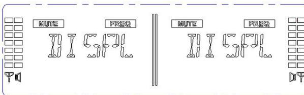
After 2-3 seconds, one of two pictures below will present: it depends on last status before turning the system off. The CPU of receiver remembers last status LCD displays what stored last time when the CPU was shut off.
