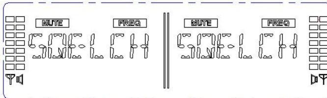
Press “SET” button and hold seconds, LCD will display Squelch like 15 dB indicates sensitivity status. Press “▲”“▼” button to change current status if need. This point is a factory pre-set at: 0-40dB. 5, 10, 15, 20, 25, 30, 35, 40dB positions are to provide optimal operation in most applications. Position at 40 dB will decrease operating range.
