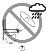
7. As shown in the figure, it is forbidden to install on the wall to prevent rain from pouring.
