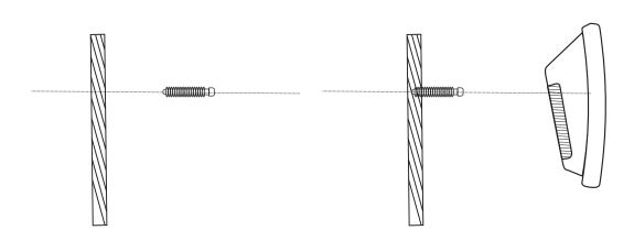
Step 1: Measured the hole in back panel by ruler. Find proper screw to fasten speaker on wall.
