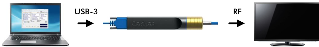
Figure 1. Typical usage of the DTU-315
