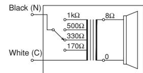
(Transformer connection when the speaker is supplied from the factory)
