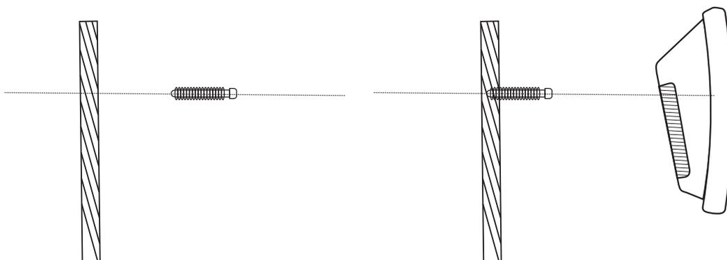
Step 1: Measured the hole in back panel by ruler. Find proper screw to fasten speaker on wall.
