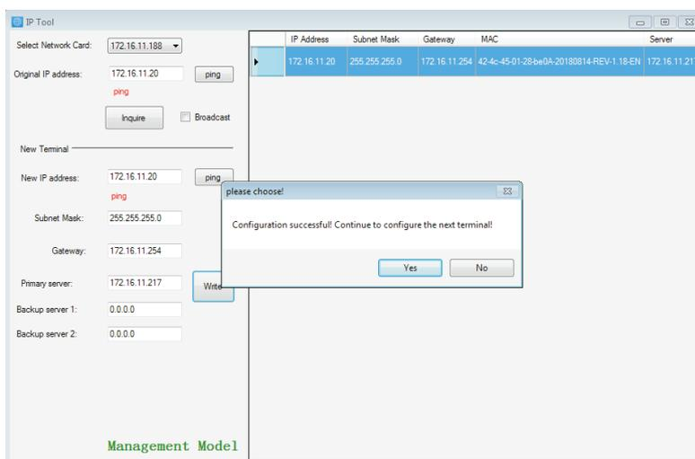
Step 5: If multiple terminals are in the same network segment, you only need to modify the IP address of one terminal, it is needed to click on the terminal in the queried terminals list, then cancel the choice of broadcast on the left interface, modify the IP address and click for configuration.
