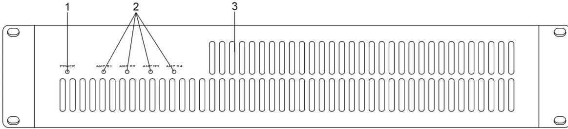
1. LED power indicator (POWER) indicates the current system power status.
