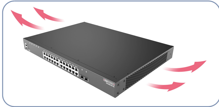
Figure 10: Switch Cooling (ECS4620-28T/ECS4620-28T-DC)
