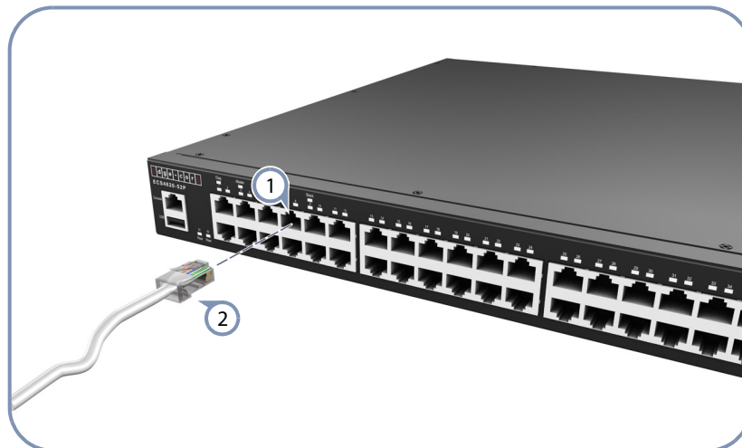
Figure 25: Making Twisted-Pair Connections
