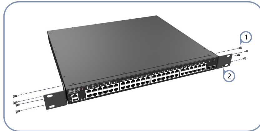
Figure 11: Attaching the Brackets
