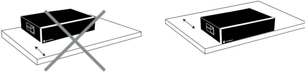
Do not place anything on top of the set-top box, instead leave a free space of 20 cm above it for proper ventilation and cooling.
