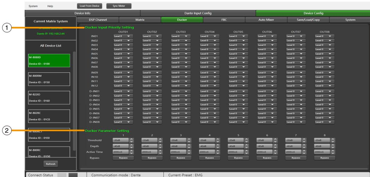
The principle of the Ducker is to attenuate one or several channels when priority signals are activated. The main applications are automatic speech for conference or priority messages.
