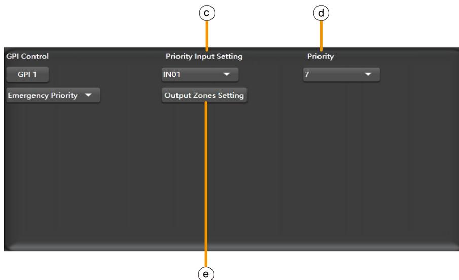
Emergency Priority is only used for emergency broadcast. This mode has higher priority than "DUCKER". When emergency broadcast is triggered, the broadcast volume setting of the corresponding channel (whether it is mute or minimum volume) will automatically return to the default volume.
