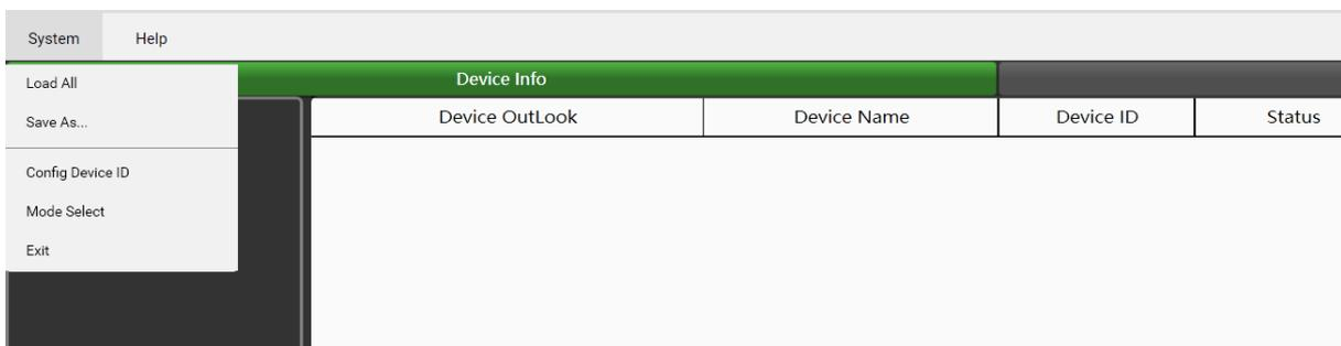
**Load All:** Load the device configuration file(except the preset list data and the Dante input configuration data).
