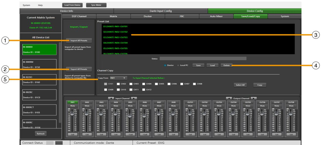
This menu is used to manage the backup parameters. These data can be stored directly in the internal memory of host as a preset. Its memory contains a total of 16 presets.
