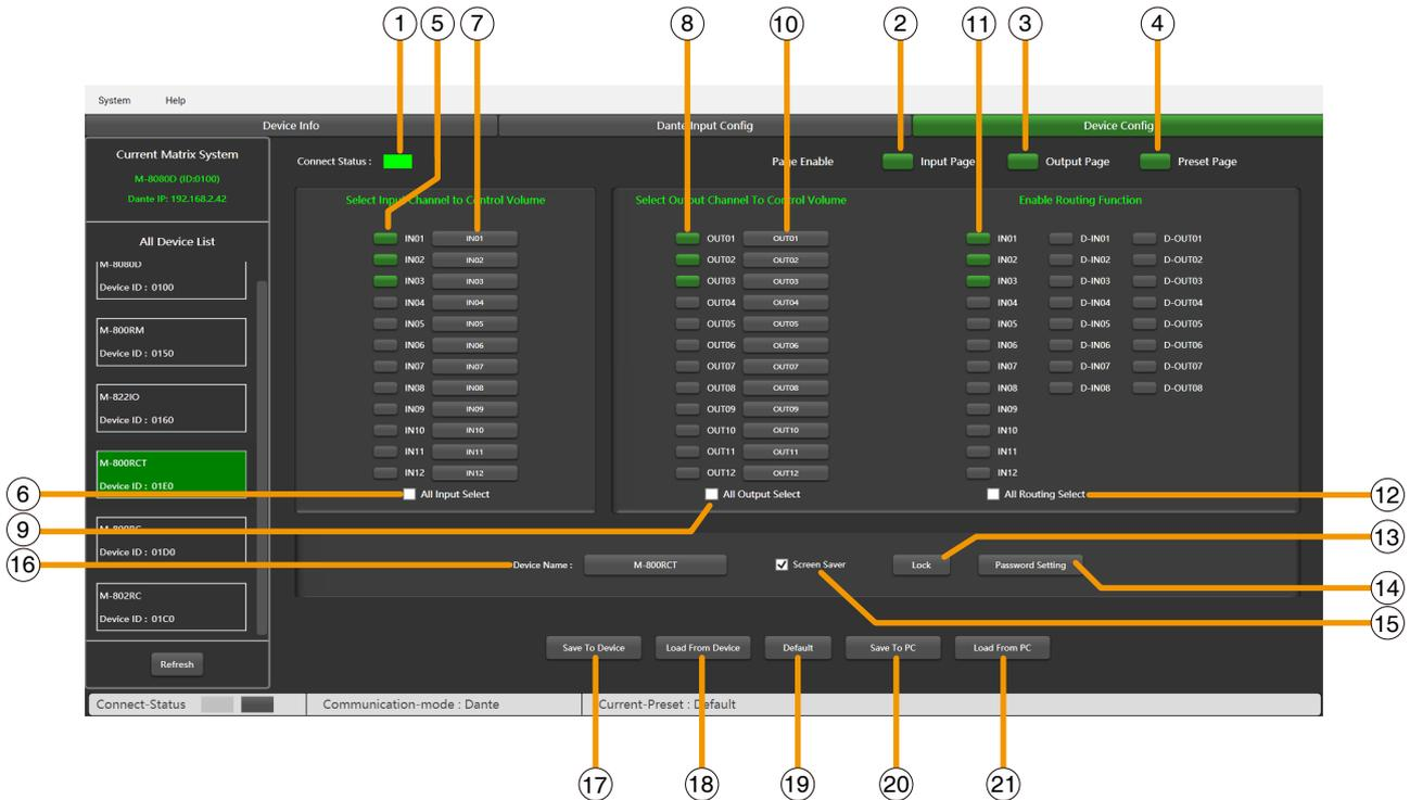
1. **Connect Status:** When the signal light shows green, it means the communication status is normal. If it shows gray, it means no communication.
