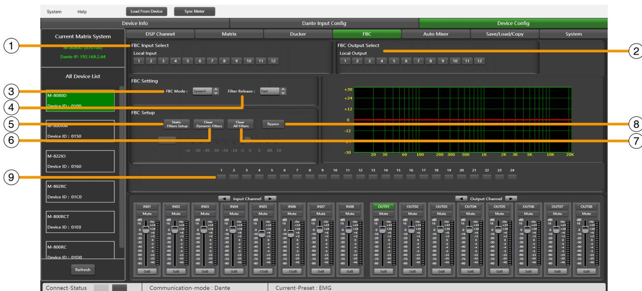
FBC (Feedback compression) function can effectively suppress howling expansion volume, ensure voice transmission quality, high fidelity, and clear sound.
