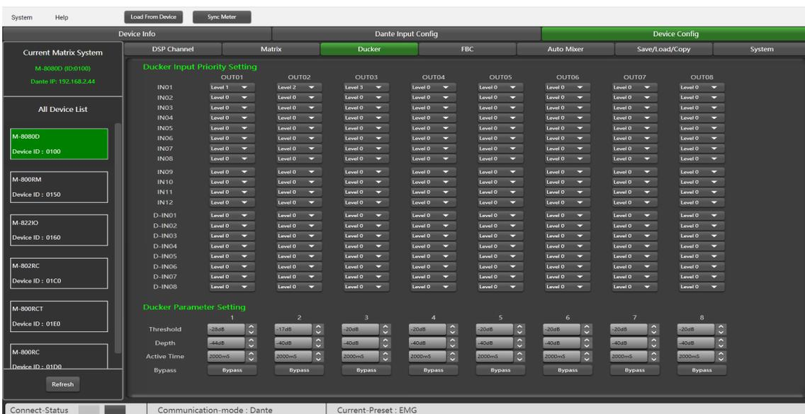
The current setting sets channel 1 to level 1, channel 2 to level 2, and channel 3 to level 3. At the same time, the Threshold, depth, and Activation Time are set at the bottom of the page. The audio source will be output according to the previously set priority and other parameters.
