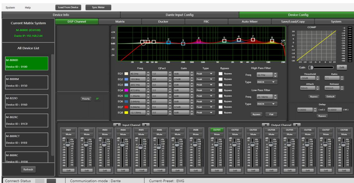
Adjust the high-pass filter / EQ point to the corresponding parameter, which is the same as Input DSP. The waveform in the EQ diagram will also change accordingly.
