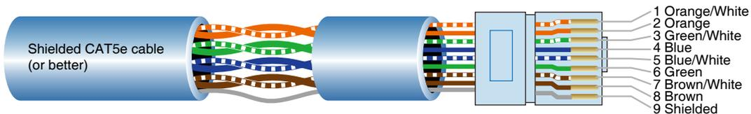
The green pair is reserved for data communications between **M-8080D** and remote device. Data communication is needed to send configuration information, software update and status information from **M-8080D** to remote device.
