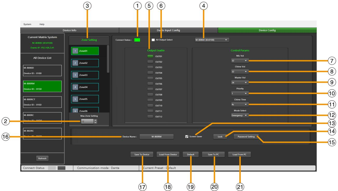
This function is a zone setting with audio routing function. You can control up to 12 output channels in a single zone. Distribute audio to different zones, and easily manage zones by adjusting the chime time / volume / priority.
