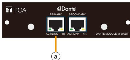
**a. LAN:** Port for the Ethernet connection, 100/1000Mbps adaptive, with DHCP function. The plug includes two LEDs, a green one indicating the good connection to the network and a yellow one indicating the good data transmission.
