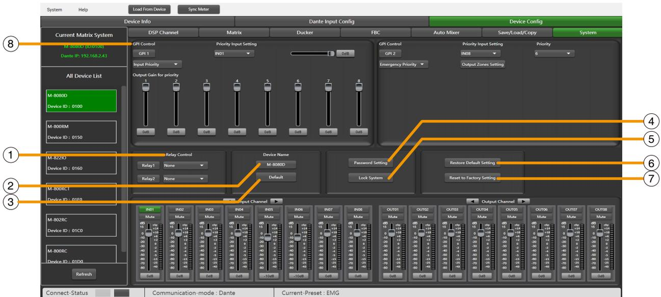
**1. Relay Control:** Either IN01-IN08 or Paging (**M-800RM**) can be selected. When there is a broadcast signal on the selected channel, the corresponding relay terminal on the rear panel of the **M-8080D** will make contact and can be used to control the start-up/shutdown of external devices.
