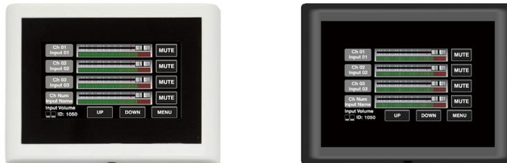
The **M-800RCT** is a wall mount 4.3" touch LC-Display volume controller. Touch LC-Display shows the volume level and the signal level for a dedicated output, the ID and communication status. It can be assigned to any output of the **M-8080D**. It can also route any input to any output like in Matrix menu of the Editor Software.
