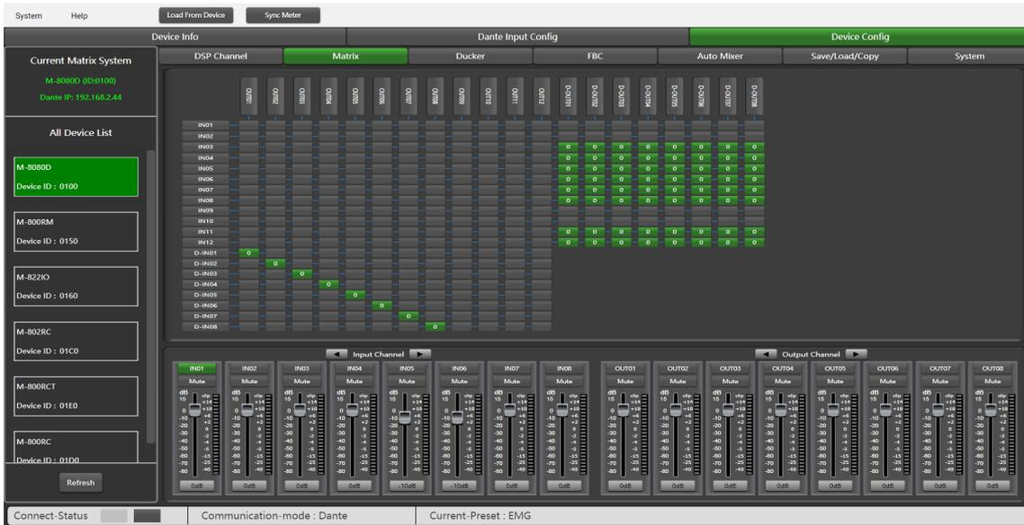
This part of the software is used to route inputs through a graphical representation as a matrix. By clicking on the gray boxes several inputs can be assigned to several outputs. If the connection is active the box turns green, otherwise it remains gray.
