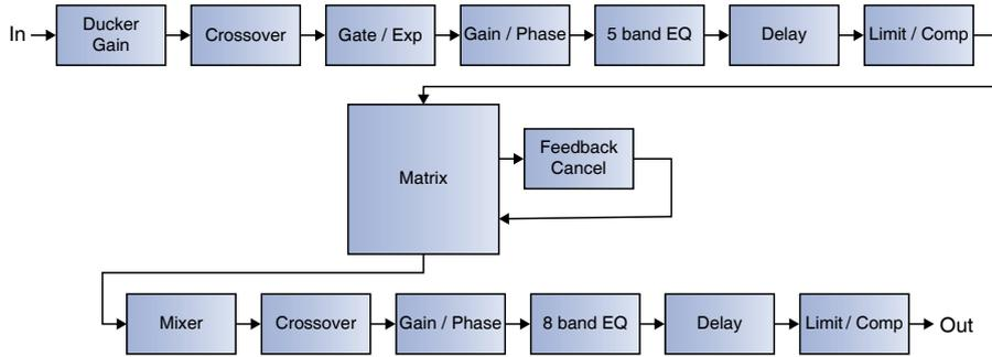
All functions can be configured with the PC Editor Software. Settings can be memorized for easy duplication or modification:
