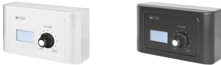
The **M-802RC** has the same functionality as the **M-800RC** volume control, but it includes 2 additional analog outputs. The device includes a built-in D/A converter processing digital audio AES3 signals from **M-8080D**. **M-802RC** requires/consumes 2x digital output channels of in total 4 available digital output channels of **M-8080D**.
