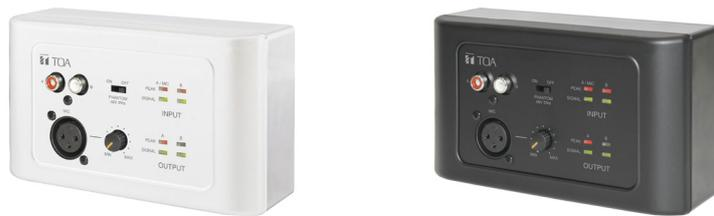
The **M-822IO** is a remote audio input and output module providing 2 x analog channels IN and 2 x analog channels OUT. The device includes built-in A/D and D/A converters processing digital audio AES3 signals from and to the **M-8080D**.
