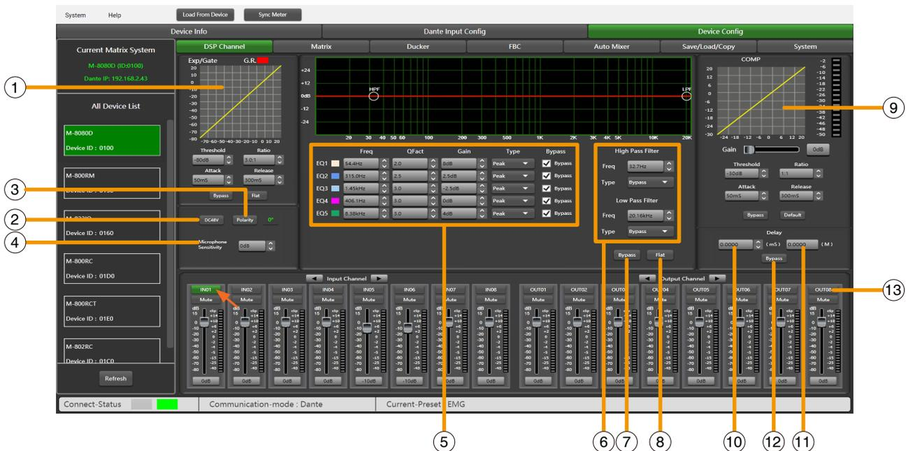
**1. EXP/Gate:** The gate attenuates signals below the threshold value, and allows signals above the threshold value to pass. When the signal is beyond the threshold, the output signal remains identical to the input signal. By adjusting the value of the ratio to its maximum, the Expander is transformed into a Noise Gate.
