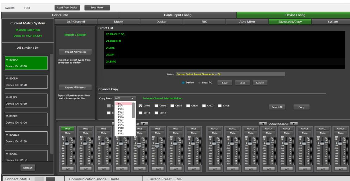
Select the input channel IN01 to copy to CH03. Click the Copy button, the parameters of input channel 01 will be copied to CH03.
