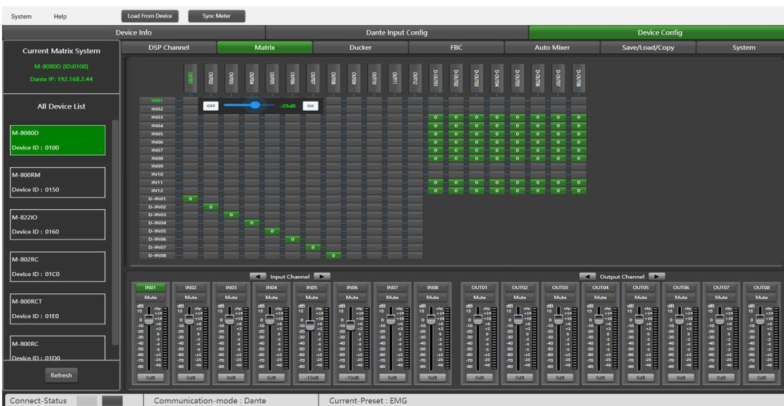
Assign input 1 to output 1: Click the Matrix node, click OFF in the pop-up window, then set the volume to -29dB, and finally click OK. The sound of channel 1 will be adjusted to -29dB.
