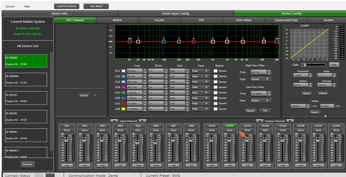
Same menu as the Input DSP Channel, without the Expander/Gate section. The parametric EQ features 8 bands here, instead of 5 bands for the inputs. Please refer to the introduction of Input DSP Channel.
