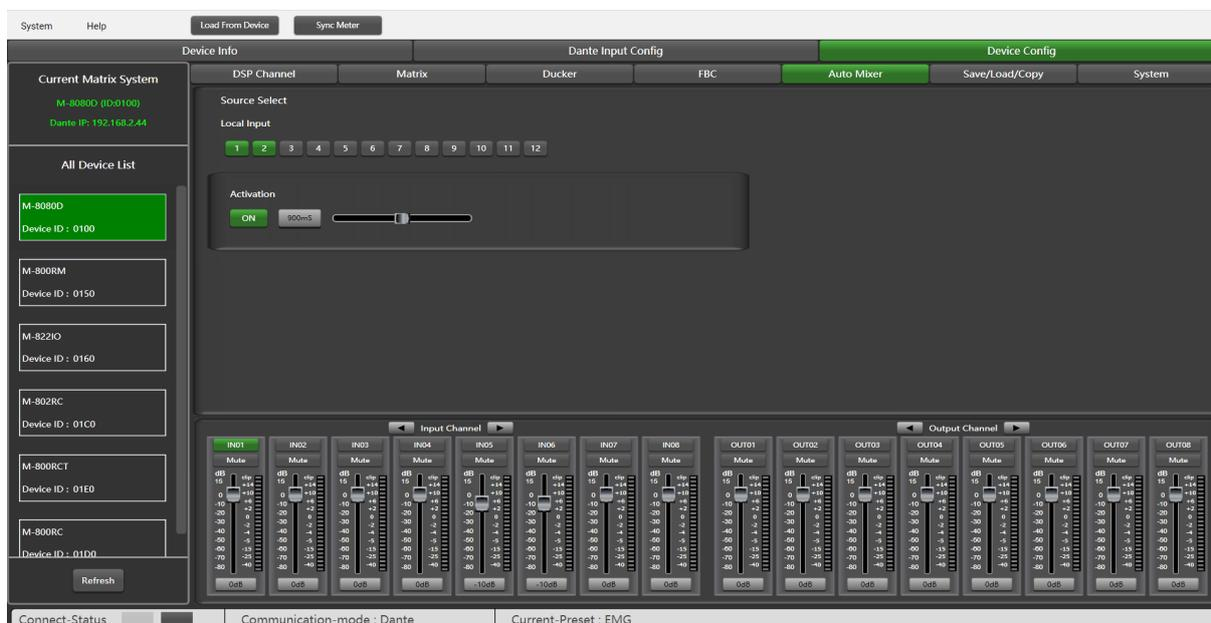
Add the local input CH 1 and CH2 open setting to the automatic mixing function. Input the audio source from two channels. Click the ON button of Active Time and push the fader to set the start mixing time of the CH 1 and CH2 signal. For example, drag the fader to 900ms, the sound source of channel 1 will be at 900ms, and the mixing function is added.
