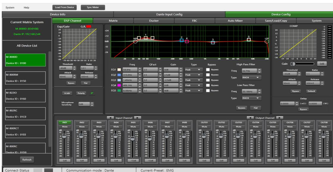
Adjusting the high-pass filter to 32.7Hz. Type is adjusted to BW24. Drag EQ1 to 54.4Hz and adjust the Q value to 2.0. Gain up to 8dB. Drag EQ2 to 315Hz. Q value is adjusted to 2.5. Gain to 2.5dB. EQ3 type to 1.45kHz The Q value is unchanged. The gain is attenuated to -2.5dB. The EQ4 type is adjusted to 406.1Hz. The Q value / gain is unchanged, and the EQ5 type is adjusted to 8.38KHz. The Q value does not change and the gain reaches 4dB.
