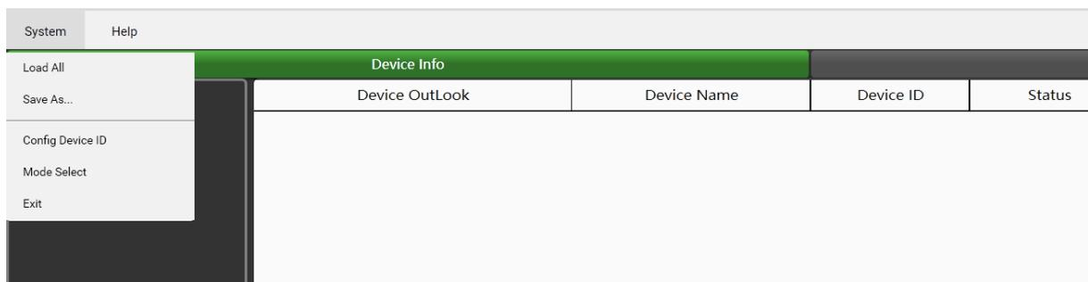
**Load All:** Load the device configuration file (except the preset list data).
