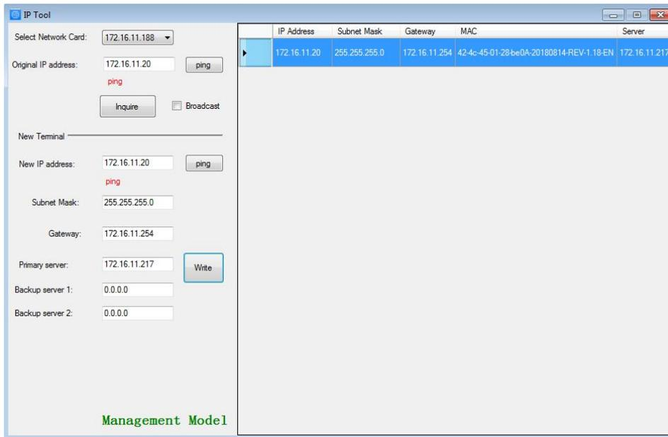
Step 4: left click on the "write" button, there will be a window prompt after the successful configuration; after that, left click on the "query" button, the parameters of the terminal will be re-read by the configuration program, if it display as the same as entered one, means that the configuration was successful.
