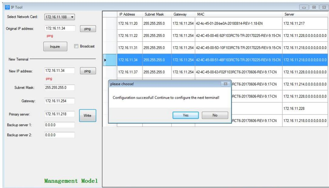
Notes: If the terminal data can't be queried or the network is blocked, the pop-up window will say Reconfigure the IP address or IP address writing error. In this case, please reconfigure the network, check the network cable, and turn off the firewall, etc.
