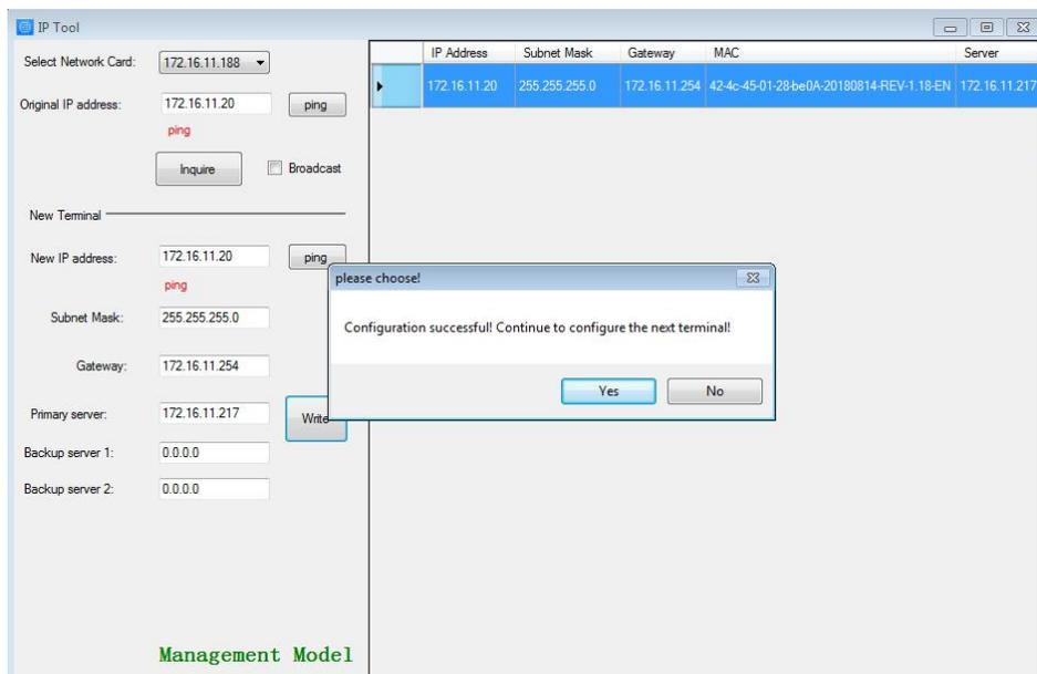
Step 5: If multiple terminals are in the same network segment, you only need to modify the IP address of one terminal, it is needed to click on the terminal in the queried terminals list, then cancel the choice of broadcast on the left interface, modify the IP address and click for configuration.
