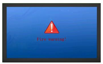
By short-circuiting the two signal pins of the ALARM output on the back of the conference controller(simulating sending a fire alarm signal to the controller), the touch screen of the conference controller and the unit device are shielded, and other functions cannot be used. When the signal pin of this interface detects that the fire alarm is canceled (the circuit is opened), it will automatically return to normal.
