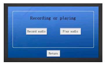
Enter the recording interface, insert a U disk, and you can play BGM or record the mixing audio of LINE IN and microphone. If there is not inserted a U disk, the interface will prompt "Please insert a U disk".
