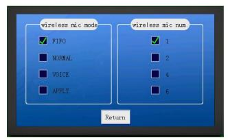
Click "Conference mode" on the main interface, select from wired/wireless mode, and then enter the wired microphone management mode. It includes 4 microphone modes and you can choose one of them; the number of microphones means the current maximum allowable number of microphones N(wired N = 1/2/4/8; wireless N = 1/2/4/6), and you can choose one of them.
