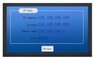
Enter the local IP interface, and you can view local IP address, gateway, subnet mask, and port number.
