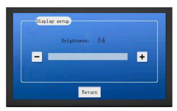
Both clicking button(+/-) and sliding the bar can adjust the screen brightness, and the adjustable range is 1~64.
