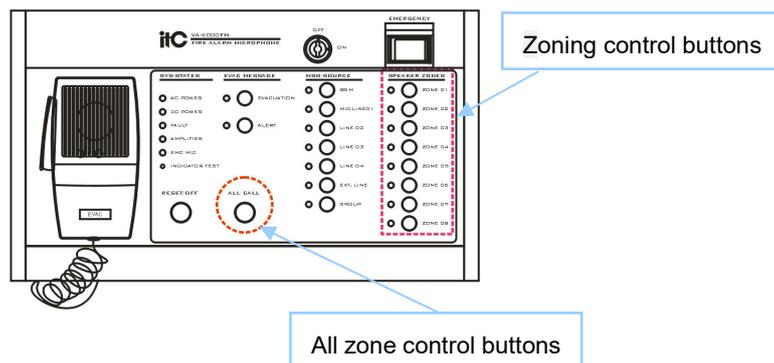
3. Press the "EVAC or ALERT" button on the VA-6000FM, the emergency system will broadcast the voice message to the selected partition or region , as shown in Figure:
