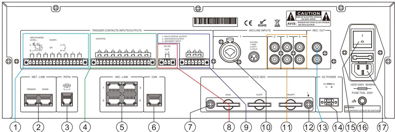
1. 8 programmable trigger input signal (which can be level signal or short-circuit signal, determined by the parameters of the machine configuration).
