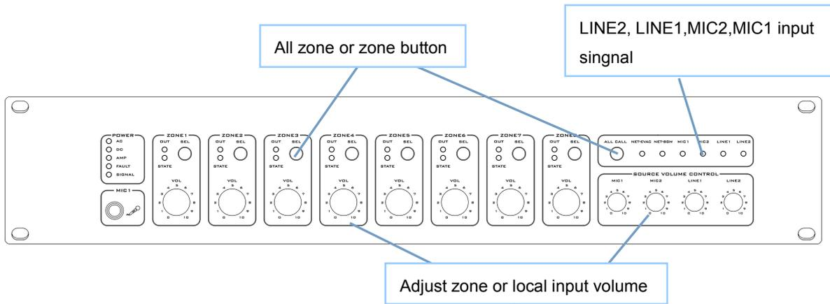
3) MIC1 emergency priority operation; when there is signal input in MIC1, the priority to output of the audio signal MIC1.
